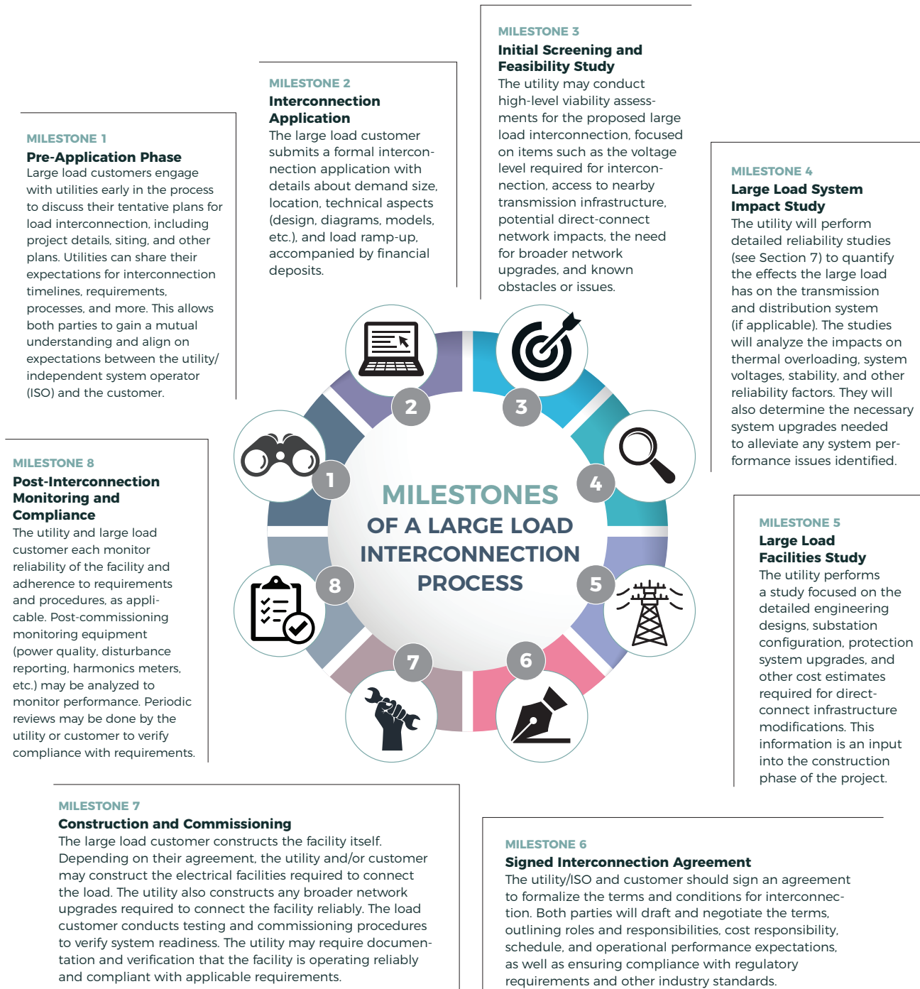
FIGURE 4.2. Milestones of a Large Load Interconnection Process
